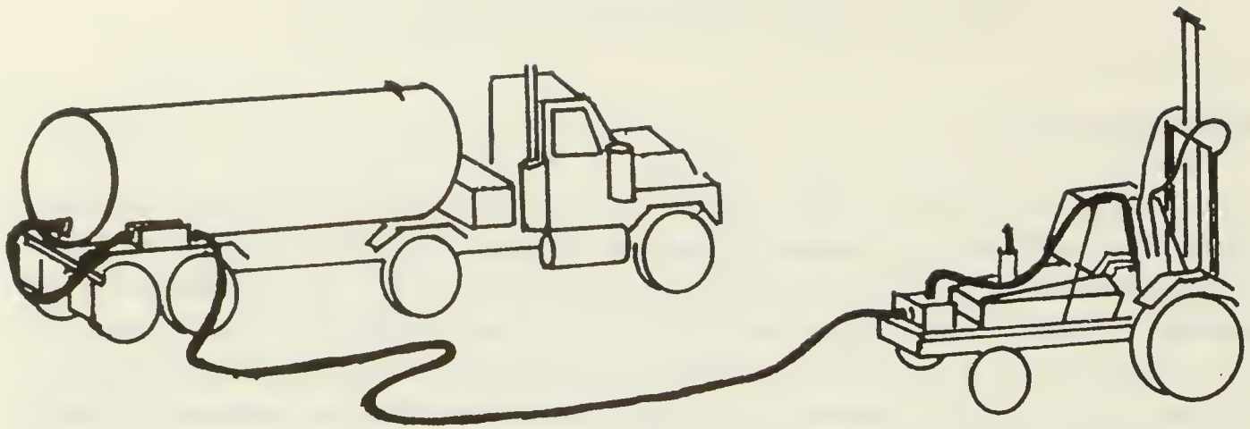
Figure 1. Illustration of slurry tank truck and injection tractor used to amend acid minesoils to the 120 cm depth.
